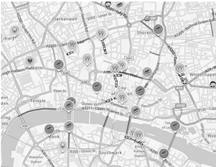
Figure 2. Screenshot taken by the author on https://www.waze.com/livemap on 5 February 2018. Shown is part of the center of London, England. The three data sources are clearly visible: the coloration of the streets is based on scraped movement data, the balloons are based on user submitted reports, and the map data comes from Google Maps.
